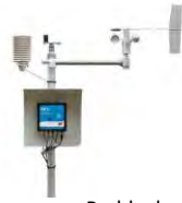
Paddock weather station providing data back to Homestead via LoRa network
