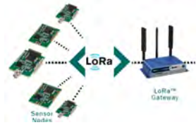
LoRa edge network, connecting in-paddock instrumentation back to the Homestead via wireless mast
