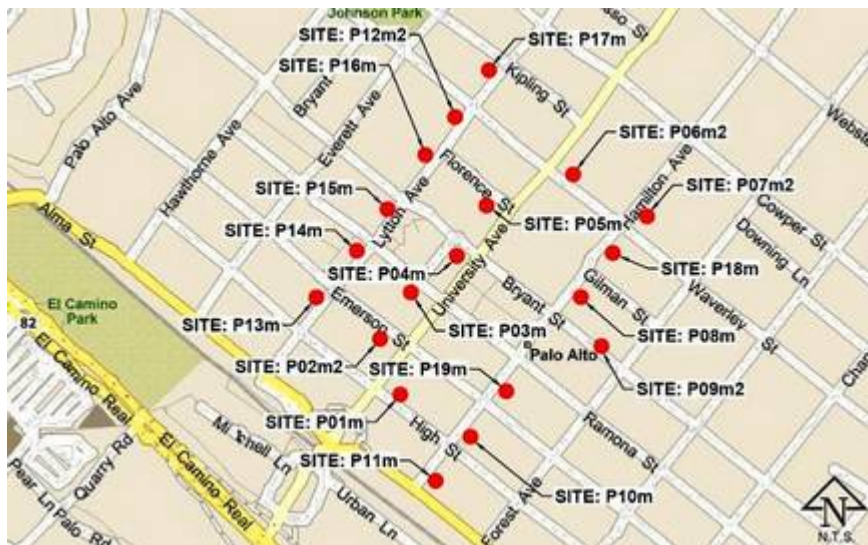
Typical small cell distribution within city commercial district.
