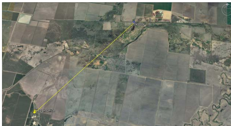
Farm and tower location rendered from Oztowers (Source: www.oztowers.com.au ) and Google Earth. (N = NBNCo, T = Telstra, O = Optus, V = VHA). Distance marker = 8.3 km
