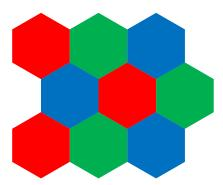
Figure 1: Illustration of 3-channel frequency reuse. Each color – red, green, or blue – represents one radio frequency.
