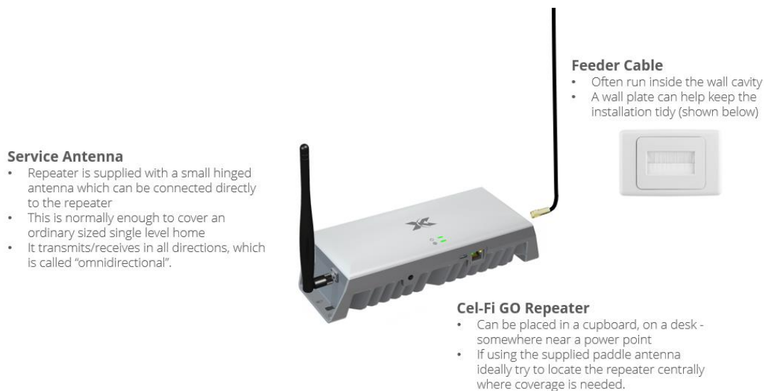
Figure 2 - Equipment inside house
