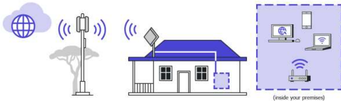
Figure 3 - Fixed wireless connection. Image: NBN
