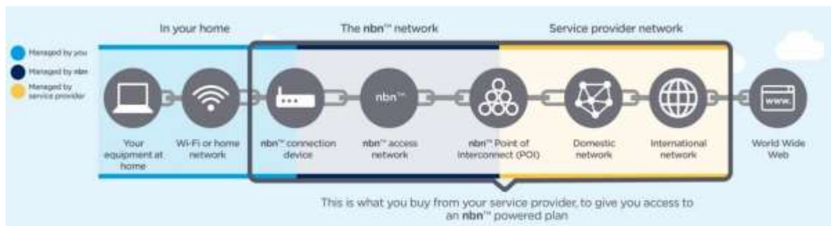
Figure 2 - How the internet works. Image: NBN
