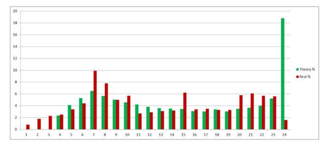
The horizontal X axis is the downstream data rate in Mb/s (as "bucketed" speeds i.e. Integer +/- 0.5 Mb/s) and the vertical Y axis is the percentage of lines at each "bucketed" speed. My first estimation of the theoretical speeds was shown by the green bars and the speeds from the analysed downloaded data (as information) were shown by the maroon bars.
