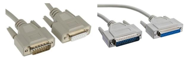
The beauty about these connectors was that they came as male and female and they consisted of two rows of parallel solder tags on the back – making them very easy to solder to multi-wire cables – and there were many connections – so there was plenty of scope to use these connectors for a very wide range of interconnecting!
