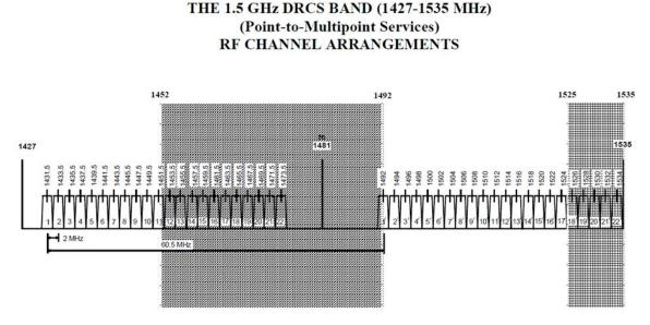
So the guard band is more like 61 MHz - 44 MHz = 17 MHz and the overall band is more like 44 + 17 + 44 MHz = 105 MHz and with this roughly centred around 1500 MHz this comes out at about 1447 MHz to 1553 MHz and the spectrum plan for this is as shown above.
