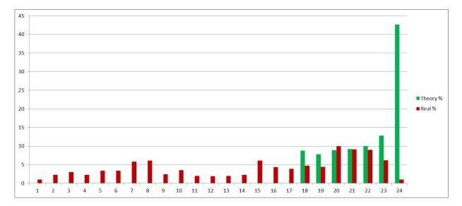
This next chart is characteristic of Large Towns, where in general the urban diameter is about 2.5 km so allowing a generous maximum urban cable length of 2030 metres (17.5 Mb/s minimum downstream speed), and makes for interesting charting. Again the Green columns are my theoretically expected results (as percentages) and the maroon columns are the percentages as grouped from the analysed reported data:
