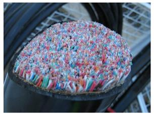
A name that sticks from TRL (J. K. Lynch) also chimed in on this innovation and developed / perfected several manufacturing techniques to significantly improve the consistency of these new plastic insulated cables. So - not only was the wire diameter far more consistent than the earlier paper insulated cables but the (plastic) insulation thickness was also to a much tighter specification.
