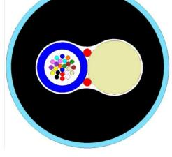
The outside diameter of this prototype cable structure would be about 15 mm to 18 mm.
