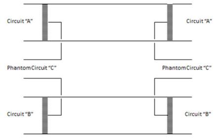
This incredibly smart innovation was that a third (loop - balanced) circuit could be derived as a "phantom" sitting over two pairs and passing its "differential" signal over each of the two other pairs in a "longitudinal" mode – then there is literally no crosstalk interference! (*You may need to read this more than once!*)
