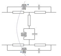
At the low frequency end of the Voiceband spectrum the attenuation was virtually the amount of the pad, (typically 6 to 12 dB). At the resonant frequency (usually somewhere between 3.5 kHz and 4.5 kHz) the attenuation was about 0.2 dB and the "B" (width) factor was a direct relation of the reactive components (to directly compensate for the shape of the "Slope" of the Access physical pair's length.
