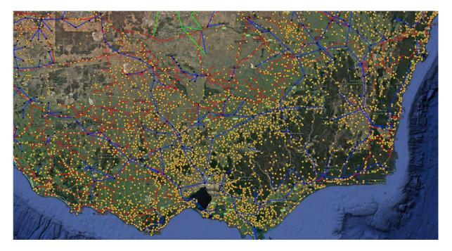
This is a map of Victoria and a bit of south NSW showing the reported Radio Black Spots as orange dots. The red lines show the paths of a high proportion of existing SMOF cables in the Regional areas, point-to-point radio hops are blue lines.
