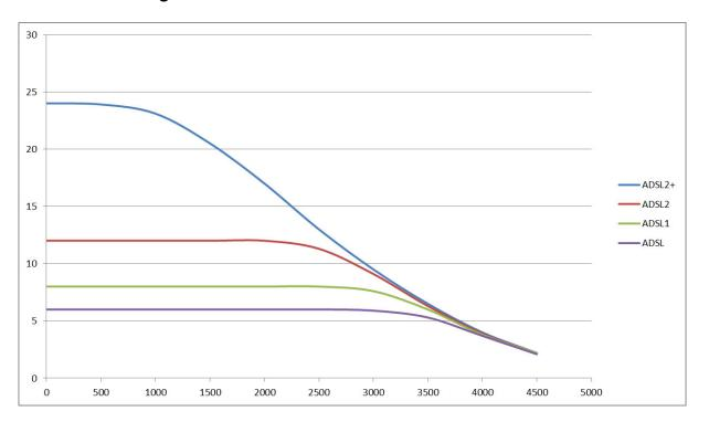
The above chart shows the theoretical downstream data speeds "y" axis (Mb/s), based on the technology of the ADSL Digital Line Services Access Multiplexer (DSLAM) versus the (0.40 mm) pair copper cable length from the Local Exchange / Node to the Customer Premises along the "x" axis (in metres).
