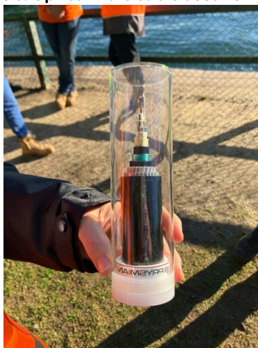
Figure 5: Optical fibre cable used for the ICF
