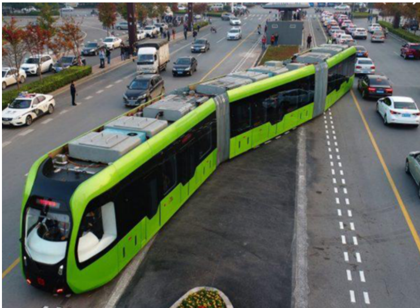
Trackless Tram currently being trialled in the City of Sterling, Western Australia.
