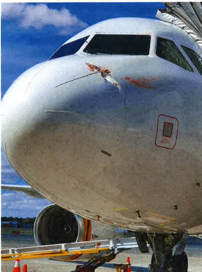
16 September 2019 – A320 Damage caused by Bird Strike at Canberra Airport
