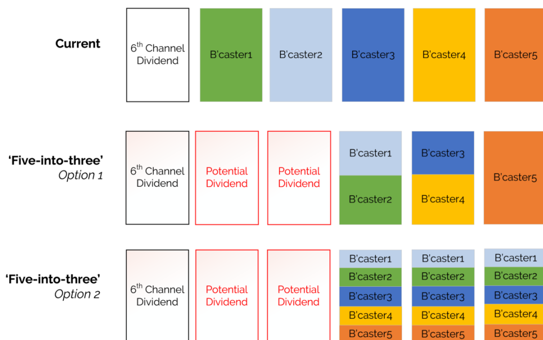
Figure 7 —Multiplex configuration scenarios: current and example 'five-into-three' options (Source: SBS)
