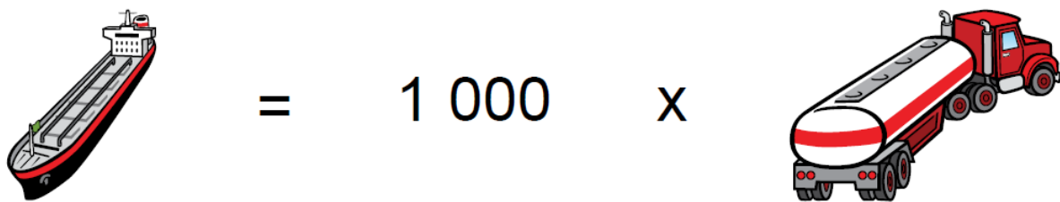
Figure 1: Volume of a Medium Range Tanker with a petroleum cargo of 30,000 tonnes compared to equivalent cargo carried by tanker truck.
