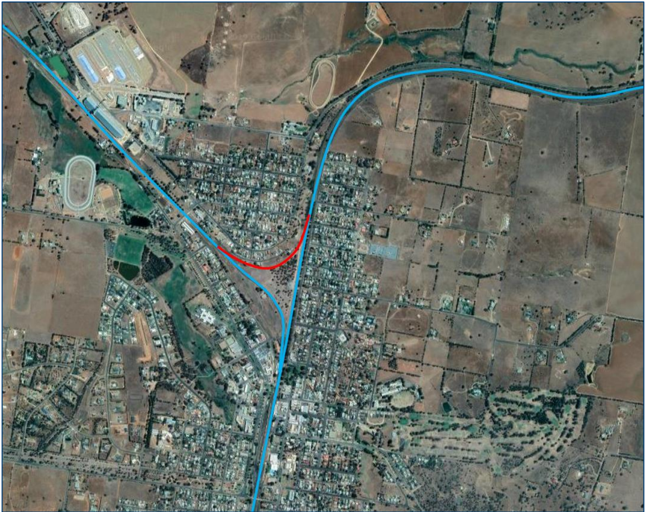
Figure 4 - Existing Lines at Junee (shown in blue) and the Proposed North Fork of the Junee Triangle (shown in red)
