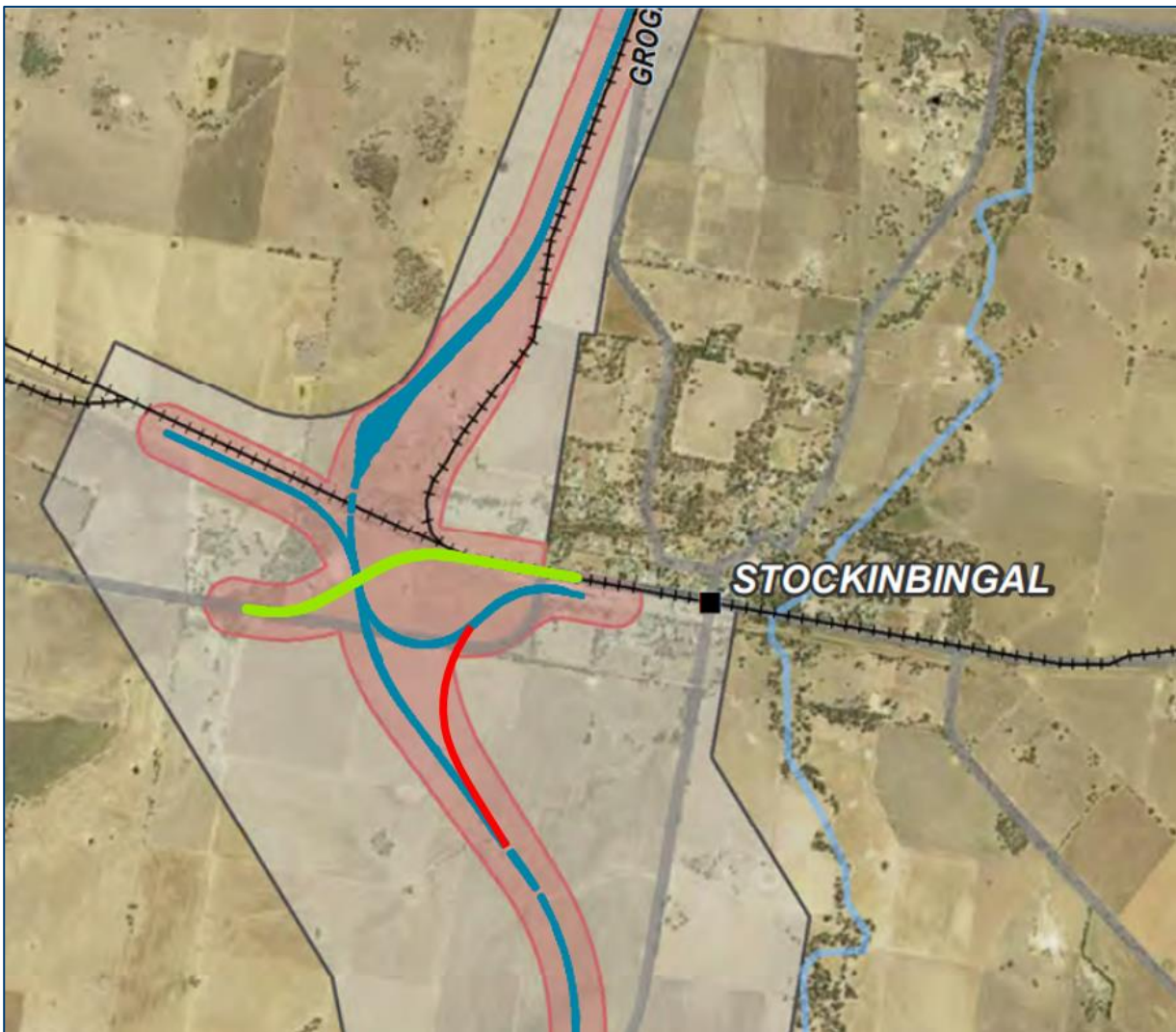
Figure 5 - South to East Connection Proposal at Stockinbingal (proposed connection shown in red, proposed Inland Rail alignment in blue, green indicates the realignment of the existing road)
