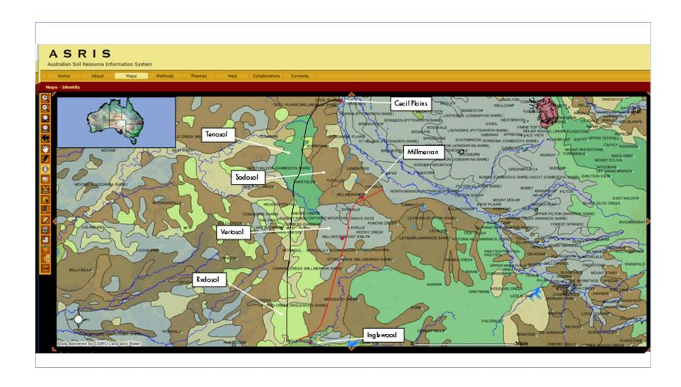
The soil type descriptions (above) clearly demonstrate the fundamental difference between the 2 different route alignments. The Cecil Plains routes follow country which is eminently suitable for heavy rail construction at base cost. The need for foundation excavation and fill with suitable material will be consequently eliminated as the soil itself lends itself to actual foundation usage.
