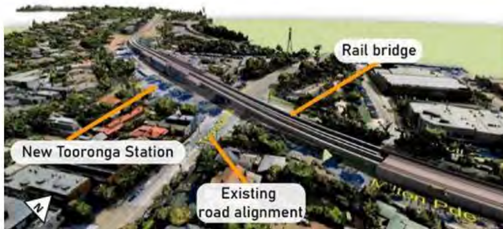
Figure 13 – Option 3: Rail over road (looking west)
