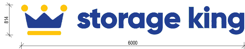
3 SIGN 3 AND SIGN 4 NON ILLUMINATED 3D SIGNAGE TO EXISTING FACADE Scale: 1:50@ A3
