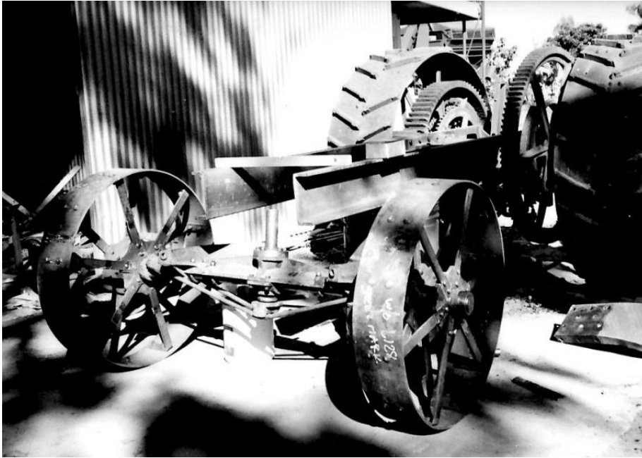
Figure 7 Titan D tractor under restoration, note the new C channel chassis rails. s22(1)(a)(ii)
