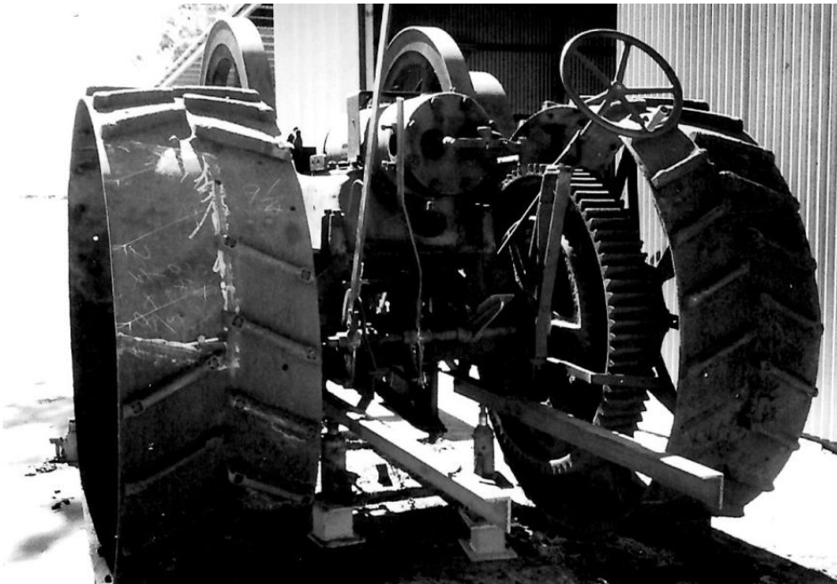
Figure 8 Titan D tractor under restoration, fitment of the rear platform support rails, and repair of missing rear wheel treads. s22(1)(a)(ii)
