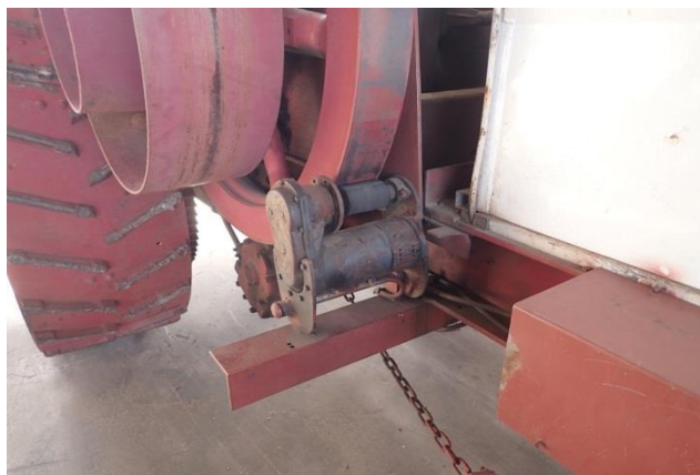
Figure 9 Electric starting mechanism, and box to the right for the battery s47F
