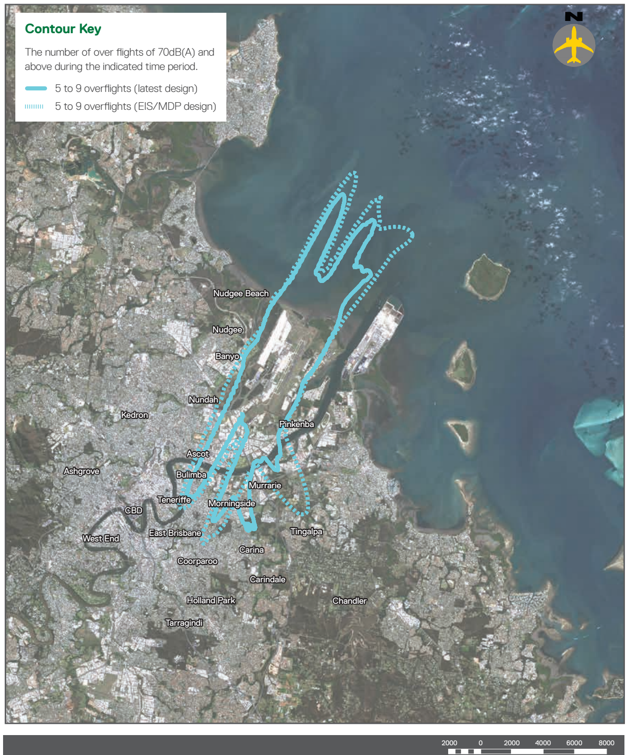
FIGURE 5: N70 CONTOUR COMPARISON BETWEEN THE LATEST DESIGN AND THE EIS/MDP - 2020 SUMMER WEEKDAY EVENING
