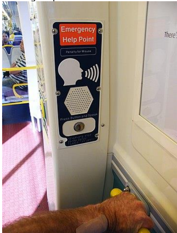
Rail car help phone not equipped with hearing loop.
