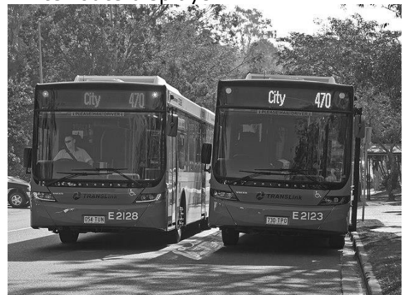
Luminance contrast of amber and white route displays.
