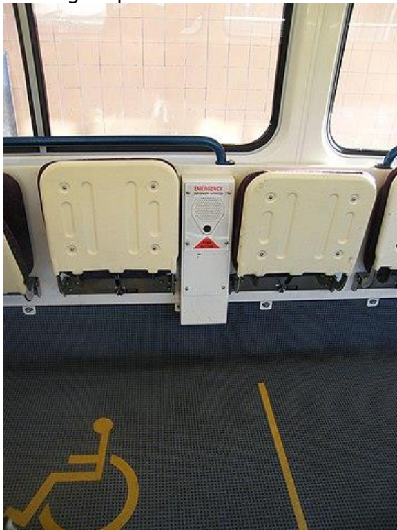
Rail car help phone not equipped with hearing loop.
