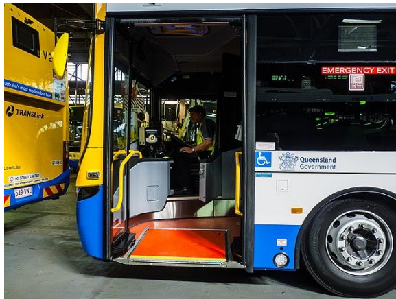
Contrasting strip and handrails at front entrance.
