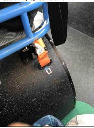
Retractable belt aisle active restraint, Queensland
