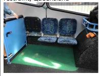
Static arm as aisle passive restraint, Germany
