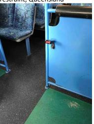
Retractable belt aisle active restraint, Queensland
