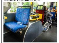
Retractable belt aisle active restraint, Queensland
