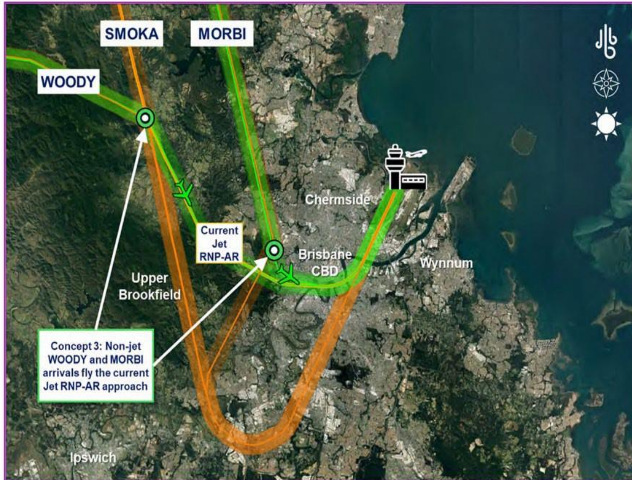
Figure 5: Example option for Concept 3 (in green with the current paths in orange) of connecting the WOODY and MORBI paths onto the existing RNP-AR over land to the new runway for suitably certified non-jet flights, when the wind is from the north
