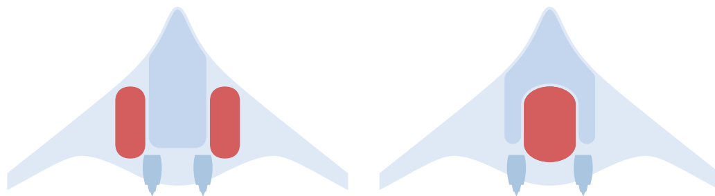
Fig. 7.2. Two potential arrangements for hydrogen tanks in a BWB configuration. The darker area shows the passenger cabin.
