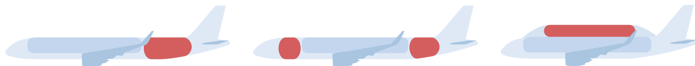
Fig. 7.1. Proposed tube-and-wing configurations store the hydrogen in the fuselage. The darker area of the fuselage shows the passenger cabin.
