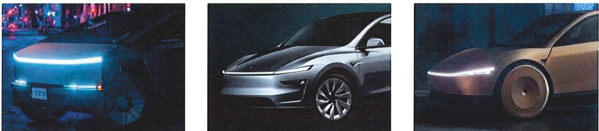
Figure 2: ADR requirements for split lights do not reflect automotive design trends
