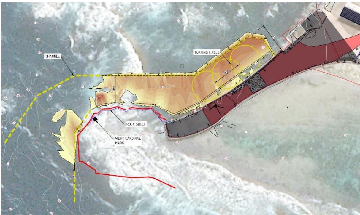
Figure 1-31 Preferred channel design alignment and volume cut.
