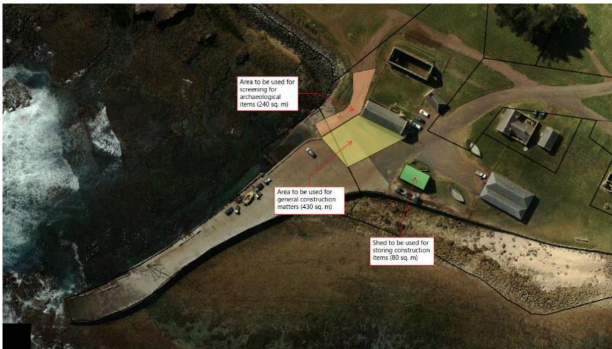
Figure 1-33 Contractor's site establishment.
