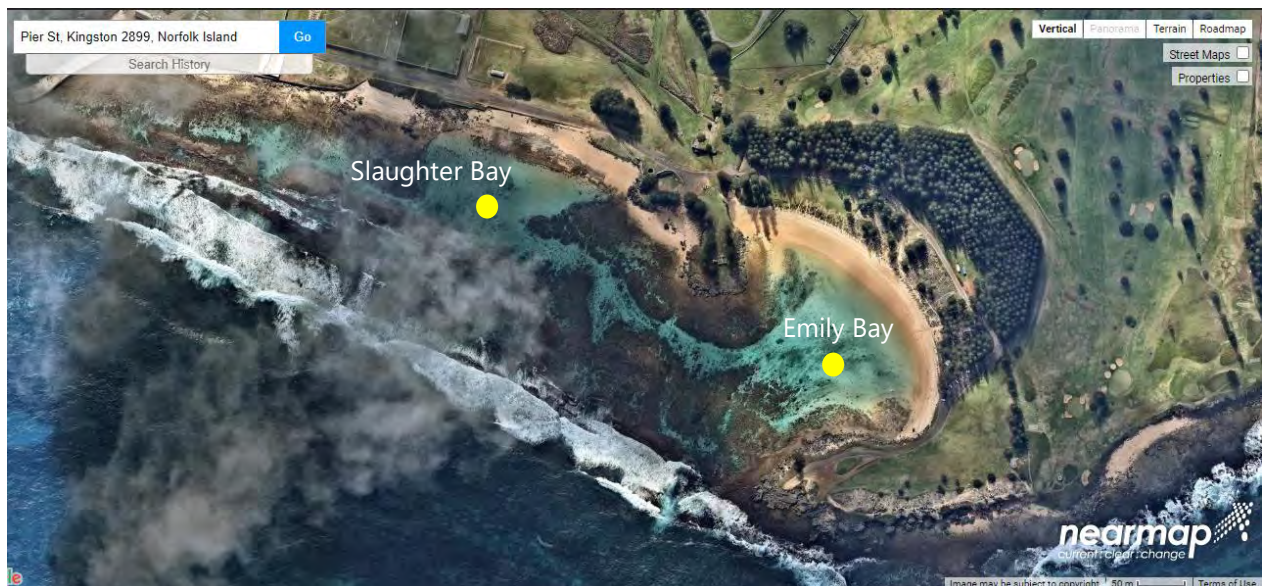
Figure 6-2 Potential turbidity baseline and construction monitoring locations (logger locations) in Slaughter Bay and Emily Bay.
