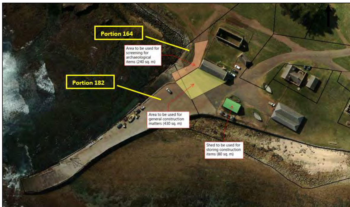
Figure 4-2 Temporary site compound at Kingston Pier.
