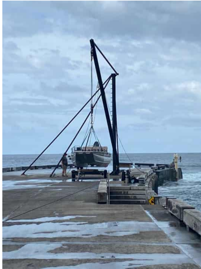
Figure 21: The dive support vessel Black Dog Cat , using derrick to launch off Kingston Pier. (Image taken 26 February 2020)
