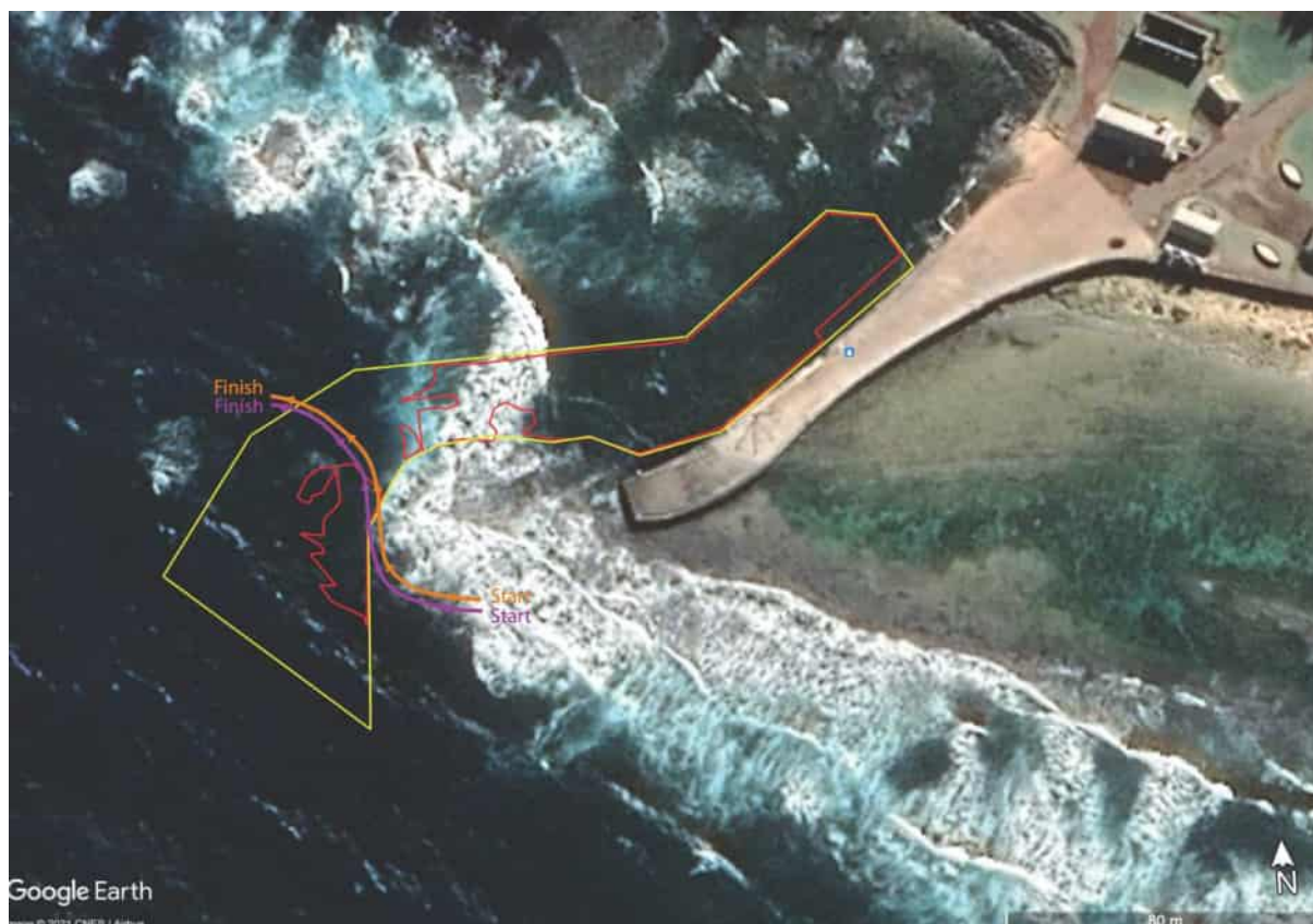
Figure 24: Video survey, inspecting seabed at proposed southern end of Kingston Pier in navigation channel. Orange track correlates with video 201117_Kingston Pier Video survey JM, purple equates to video 201117_Kingston Pier Video survey JB. (Base image Google Earth).
