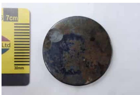
Figure 37: Object ID:0189, metallic engine tappet shim. Material unidentified, non-ferrous/magnetic.
