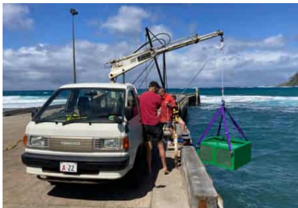
Figure 18: Method of extracting sediment boxes using a small crane truck. (Image taken 8 November 2020).
