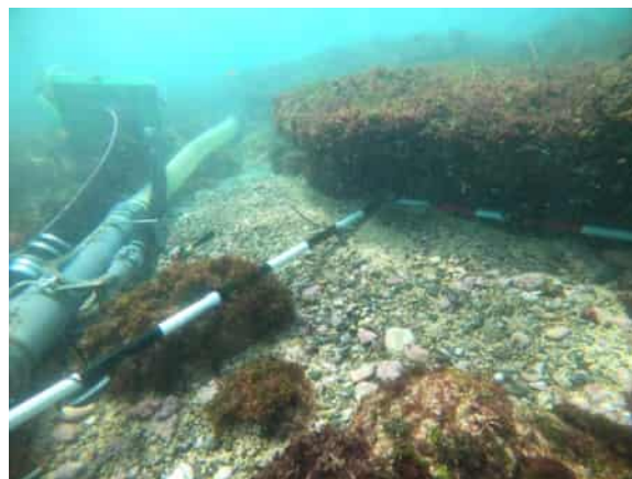
Figure 51: Sediment in TT4 was a sand matrix with cobbles. Image facing SW. (Image taken 12 November 2020).
