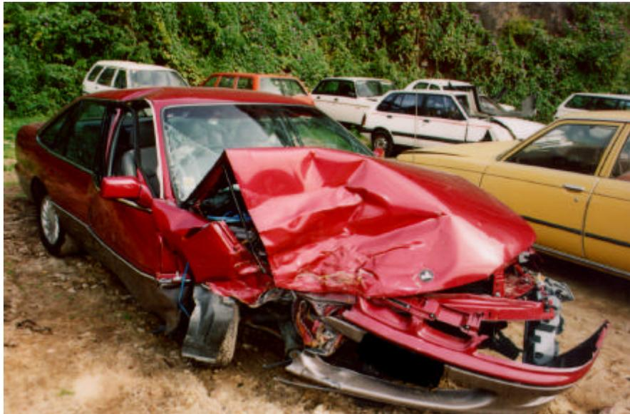
*Figure 3.1 Offset Frontal Impact -Collision Direction of Force is 12 o'clock*
